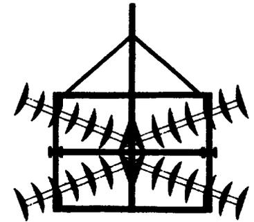
**Figure 1. Disk gang angle.** that more residue remained on the surface when operating depth was 4 and 6 inches than when depth was 8 or 10 inches. Percentage of residue remaining was about constant at field speeds of 4.5 to 6 miles per hour (mph), but increased when field speed was lowered to 1.5 mph.
